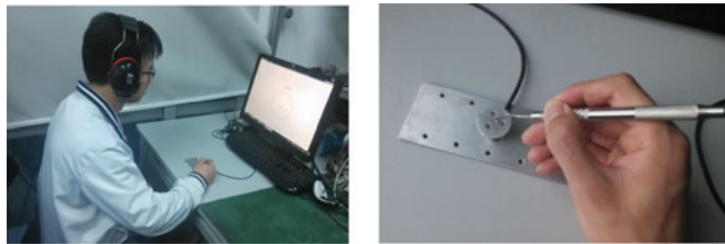
Fig. 1. Experiment system. a) A participant in test. b) Detailed view of pressing the probe on the force sensor.
