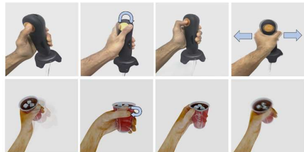
Figure 12: Gestures and their corresponding haptic feedback in the VR scene. (a) grabbing and release objects (b) rubbing with the thumb to feel textures, (c) squeezing and pressing to feel the softness, (d) shaking to feel vibrations.
