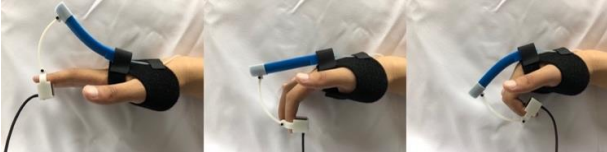
Fig. 14. Measuring fingertip forces during repeated grasping motion
