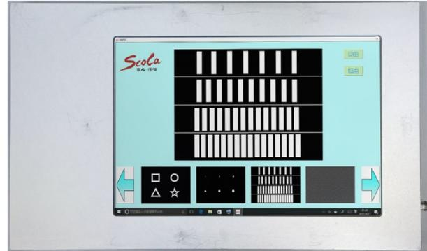
Figure 5. Custom-designed electrostatic tactile display device used in this study, described and validated in our prior research [31].
