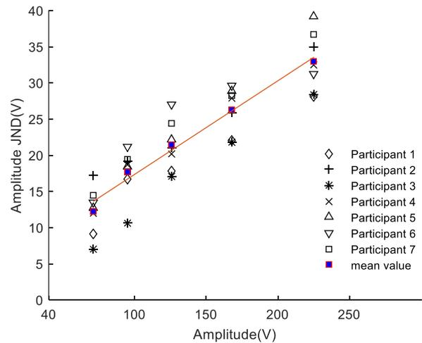
Figure 5 JNDs of the voltage amplitude at 169Hz for all participants and the mean value.
