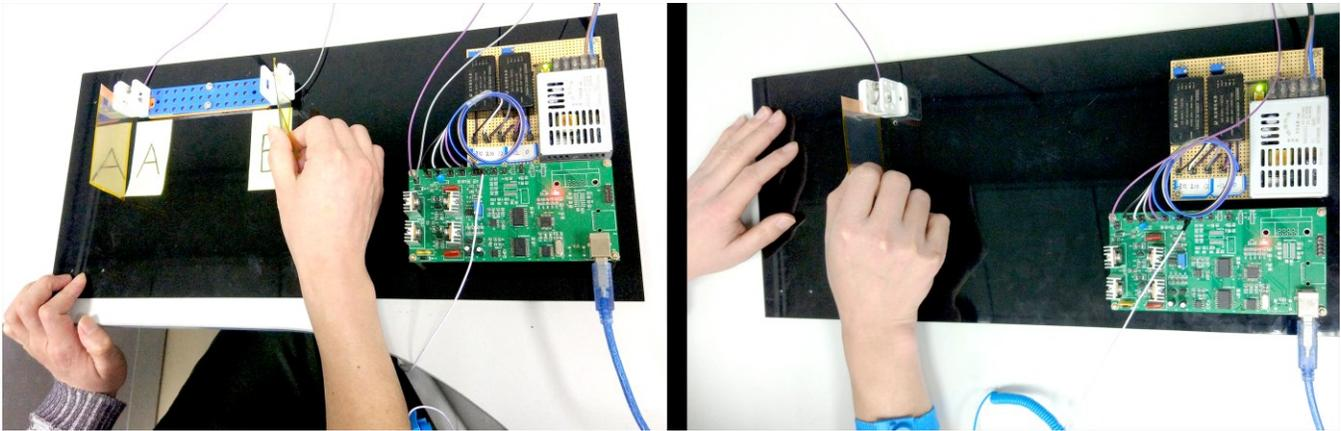
Figure 2 Experimental setup testing absolute detection thresholds(left) and JNDs of voltage amplitude at the most sensitive frequency(right).
