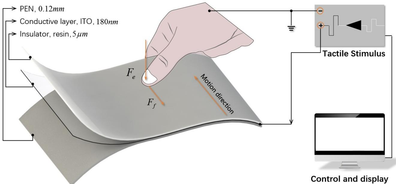
Figure 1 FlexTouch operating principle. The controller generates the changing voltage.
