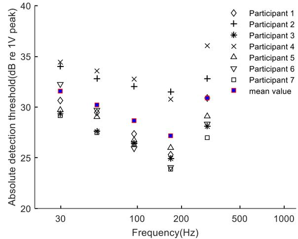
Figure 4 Mean absolute detection threshold of FlexTouch.
